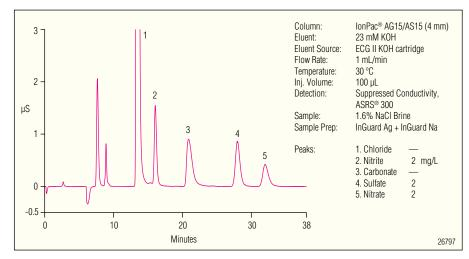
Figure 2. Analysis of 2 ppm nitrite, nitrate and sulfate in 1.6% NaCl Brine after on-line sample pretreatment with InGuard Ag and InGuard Na cartridges.
