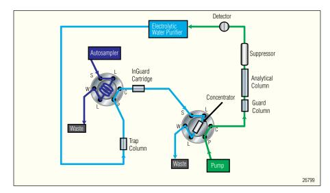
Figure 4. Preferred configuration 2: two 6-port valves, one pump, and an Electrolytic Water Purifier.
