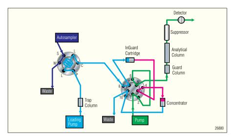
Figure 5. Preferred configuration 3: one 6-port and one 10-port valve, and two pumps with stopped flow.
