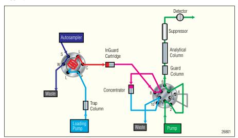
Figure 6. Preferred configuration 4: one 6-port and one 10-port valve, and two pumps with constant wash.
