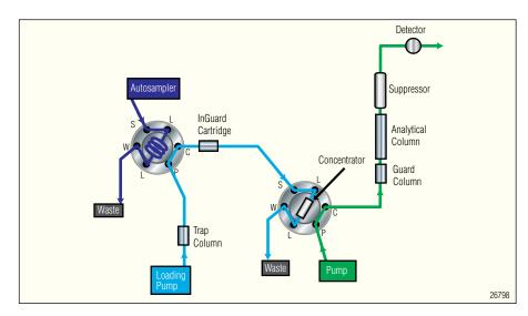
Figure 3. Preferred configuration 1: two 6-port valves and two pumps.
