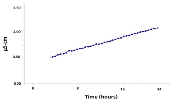
Figure 2a. Measured carbonate (peak height) by anion RFIC in deionized water (20 hours).
