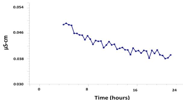
Figure 2b. Measured carbonate (peak height) by anion RFIC in iWP water (20 hours).
