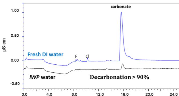
Figure 1: Comparison of deionized water and Trovion *iWP* water. (Conditions: Dionex AS18 separator (4 mm), 25 mM KOH @ 1.0 mL/min, ASRS®)
